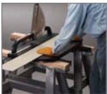
A 90° guillotine fence is quickly installed to the left or right of blade for cutting siding planks to length.
