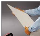
Scribe desired angle on fiber cement siding plank and feed it into the guillotine blade as you cut.
