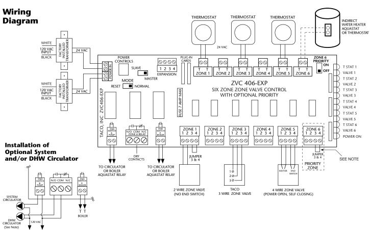
**Operation/External Diagnostics:** When any thermostat calls for heat, the appropriate zone valve is energized and the yellow light goes on. When the zone valve is fully open, the red light goes on and energizes the end switch relays. The green light should always be on, indicating that power is connected.
