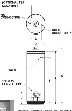
Maximum Hydrostatic Working Pressure: 150 PSI.
