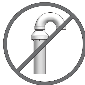
Figure 5-5 Do Not Install U-Bend to Rain Cap
