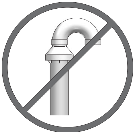
Figure 5-5 Do Not Install U-Bend to Rain Cap
