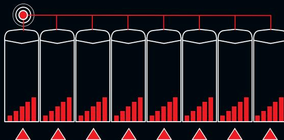
This feature optimizes the modulation capabilities of the Boiler Plant while evenly distributing run time across all cascaded boilers. Every 24 hours the SMART SYSTEM automatically shifts the 1st boiler on role to the next in the sequence, distributing run time equally.
