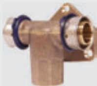
Viega ProPress Tee Zero Lead - For fire sprinkler systems - Only use with ViegaPEX Ultra tubing Model V5009.1,V5009.51 - Bronze - Press connection, female pipe thread - Mounts to vertical surfaces Note For use with black ViegaPEX Ultra only. UL listed for NFPA 13D systems Model 2818.3ZL
