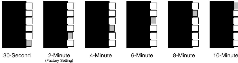
**NOTE: SELECT ONLY ONE DIPSWITCH CORRESPONDING TO THE DESIRED FEED DELAY.**
