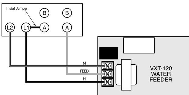
**ALTERNATE WIRING:** If you choose to wire the feeder to a separate power source from the burner circuit, do not install jumper between L1 and A. Connect a wire from the "Feed" terminal on the water feeder to terminal A on the low water cut-off. Connect a wire from terminal H on the water feeder to the hot side of the power source. Connect a second wire from terminal H to the other terminal A on the cut-off. Connect a wire from terminal N to the neutral side of the power source.
