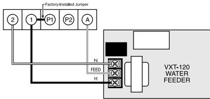
**ALTERNATE WIRING:** If the power source for the low water cut-off is separate from the burner circuit (indicated by the absence of a jumper between terminals 1 and P1 on the low water cut-off), connect a wire from the "Feed" terminal on the water feeder to terminal A on the low water cut-off. Connect a wire from terminal H on the water feeder to burner circuit hot. Connect a wire from terminal N on the water feeder to burner circuit neutral.
