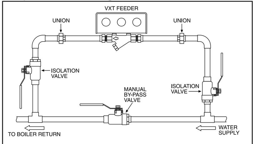
Feeder must be installed with a manual by-pass. Use isolation valves and unions to allow easy removal for service or replacement.
