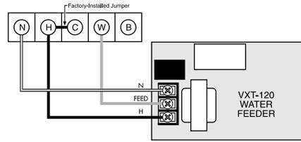
**ALTERNATE WIRING:** If the power source for the low water cut-off is separate from the burner circuit (indicated by the absence of a jumper between terminals H and C on the low water cut-off), connect a wire from the "Feed" terminal on the water feeder to terminal W on the low water cut-off. Connect a wire from terminal H on the water feeder to burner circuit hot. Connect a wire from terminal N on the water feeder to burner circuit neutral.
