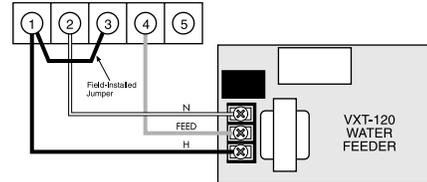
**ALTERNATE WIRING:** If the power source for the low water cut-off is separate from the burner circuit (indicated by the absence of a jumper between terminals 1 and 3 on the low water cut-off), connect a wire from the "Feed" terminal on the water feeder to terminal 4 on the low water cut-off. Connect a wire from terminal H on the water feeder to burner circuit hot. Connect a wire from terminal N on the water feeder to burner circuit neutral.
