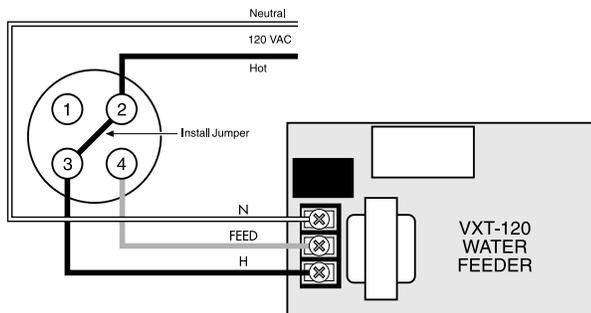
**ALTERNATE WIRING:** If you choose to wire the feeder to a separate power source from the burner circuit, do not install jumper between 2 and 3. Connect a wire from the "Feed" terminal on the water feeder to terminal 4 on the low water cut-off. Connect a wire from terminal H on the water feeder to the hot side of the power source. Connect a second wire from terminal H to terminal 3 on the cut-off. Connect a wire from terminal N to the neutral side of the power source.
