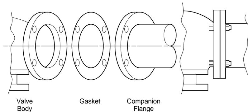
Figure-5 Installation of Flanged End Valves.
