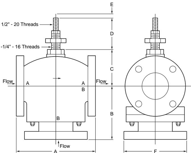
Figure-10 Typical of VB-9313-0-5-P, 2-1/2" to 6" Valve Bodies.
