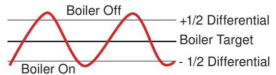
In order to decrease temperature swings and increase boiler efficiency, the Auto Differential feature automatically adjusts the operating differential of the boiler based on the heating load. As the load increases, the differential will decrease to minimize temperature swings. As the load decreases, the differential will increase to prevent short cycling. This can significantly improve operating efficiency and prevent equipment failures through excessive cycling.
