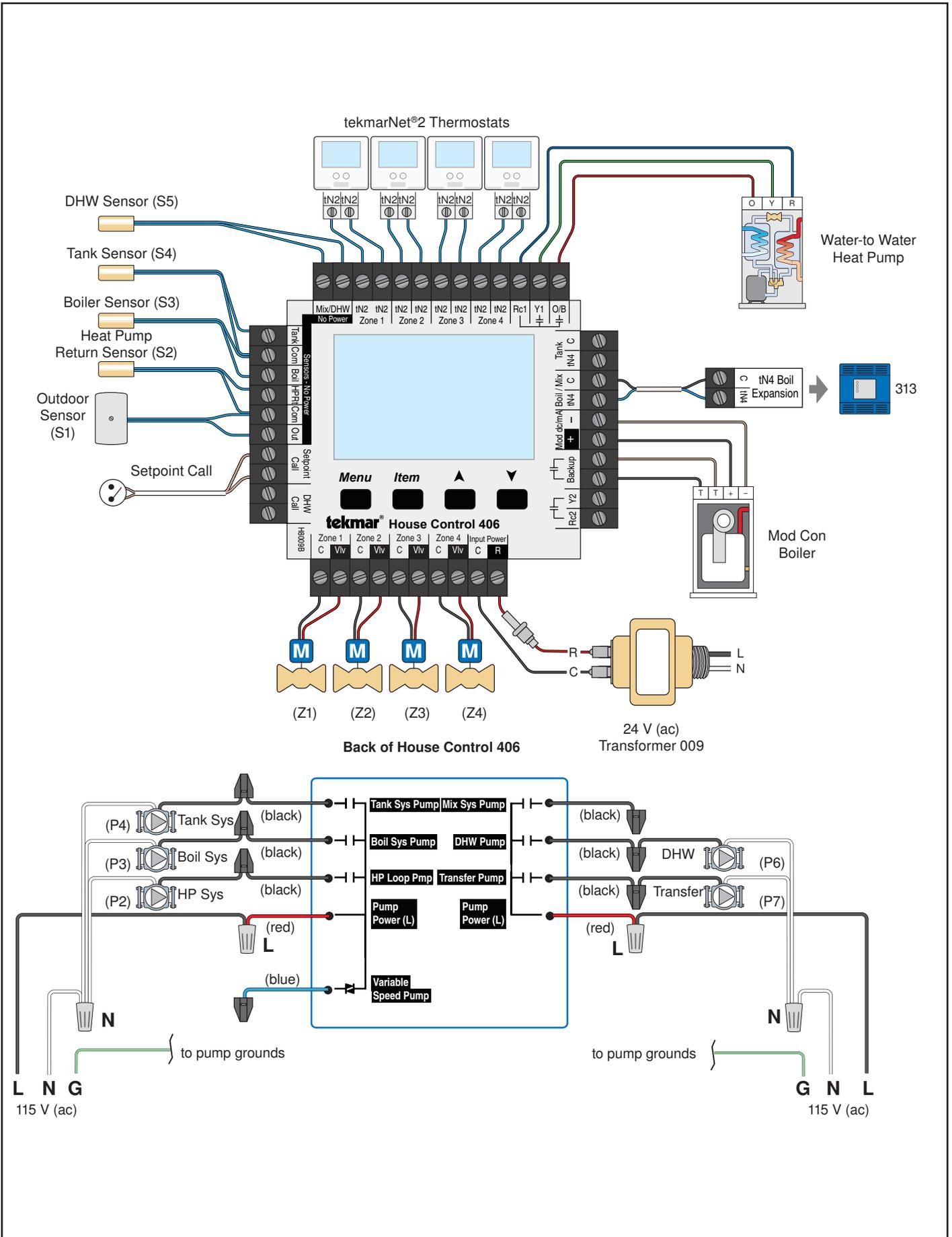
**Description:** The House Control 406 operates a two stage water source heat pump in heating or cooling mode to supply an outdoor reset water temperature to 4 on board tank temperature zones. The 406 also operates an on/off boiler to supply an outdoor reset water temperature to 4 boiler zones connected to the Boil expansion terminals with a Wiring Center 314. The boiler supplies backup heat to the tank loop using the variable speed pump P1.
