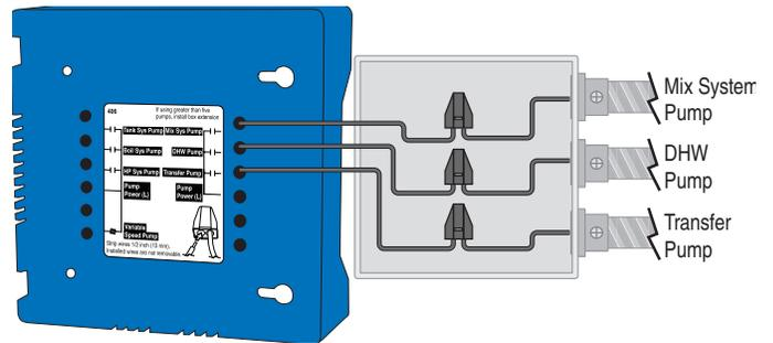
**Rear Line Voltage Wiring Diagram**
