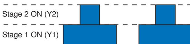
With a geo source heat pump selected, the 406 will stage on sequentially, but turns off both stages at once. This allows the ground to naturally recover better since there are longer periods of time between the heat pump transferring heat to or from the ground source.
