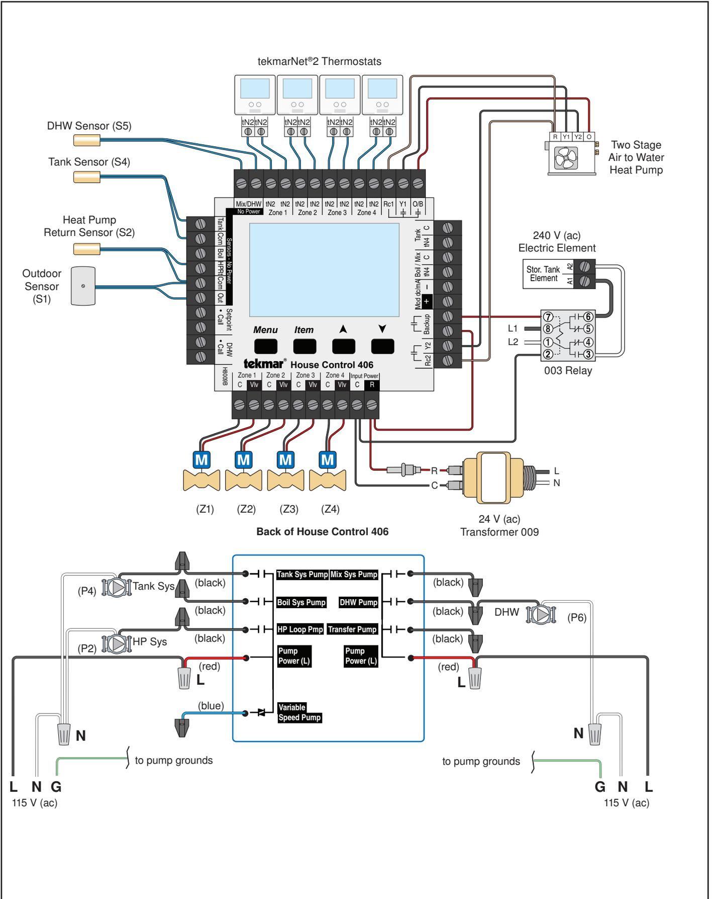
**Description:** The House Control 406 operates two air source heat pumps in heating or cooling mode to supply an outdoor reset water temperature to 4 on board mix temperature zones and 4 tank zones connected to the Tank expansion terminals with a Wiring Center 314. An electric boiler supplies backup heat using the Backup relay and the Transfer Pump P7.
