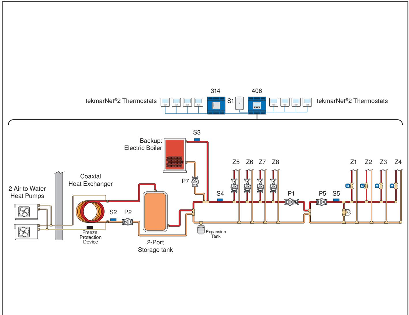
**Description:** The House Control 406 operates a water source heat pump in heating or cooling mode to supply an outdoor reset water temperature to 4 on board tank temperature zones. The 406 also operates a modulating condensing boiler to supply an outdoor reset water temperature to 4 boiler zones connected to the Boil expansion terminals with a Wiring Center 313. The boiler supplies backup heat to the tank loop using the transfer pump P7.
