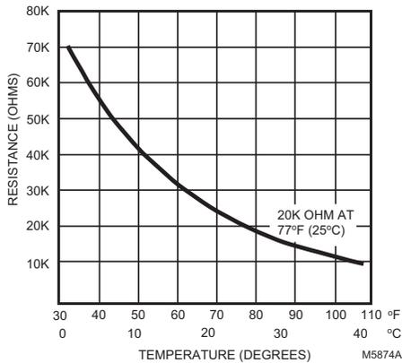
Fig. 1. Temperature vs. Resistance for Nonlinear Sensor.
