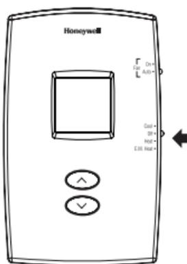
Use the **System** switch to place the system in one of the following modes.
