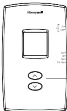
Press the ^ or v button once to display the setpoint temperature. Press either button more than once to change the setpoint.
