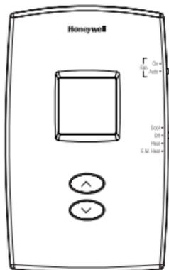
Use the **Fan** switch to select the fan operation.
