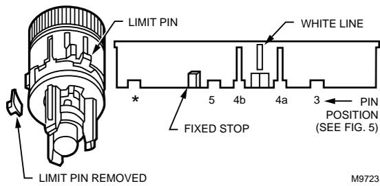
5. To replace the adjustment knob, align the knob setting from step 3a with the white line on the base and push the knob toward the base. Make sure the three arm clips snap in place at the top of the adjustment knob.
