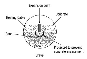
ProMelt must be embedded in a sand bed when transitioning out of the concrete slab.
