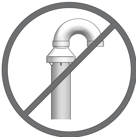
Figure 4-5 Do Not Install U-Bent to Rain Cap
