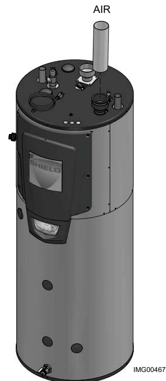
Figure 2-6 Near Water Heater Air Piping
