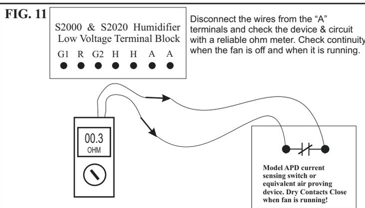
The latest improvement to the Field Controls humidifiers is the new "Airflow Interlock Feature" provided on the low voltage terminal block. Due to popular demand we have made it easier for you to achieve fail safe lockout in the event the fan or blower on the HVAC system does not operate when called upon. A high humidity or airflow proving device is necessary.
