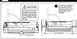
1. FOR THE RIGHT REAR PIPING Right Rear piping Step-2 Install the Indoor Unit r**O** • Step-3 Secure the Indoor Unit Step-4 Insert the connecting cable In case of the cover is cut, keep the cover at the rear of chassis as shown in the illustration for future
