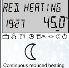
Continuous reduced heating and reduced hot water operation according to set back temperature set point
