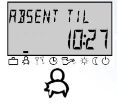
Absent / Economy setback-Heating will be inactive until specified time (this example is 10:27 am). This can be set between 0.5-24 hours OR if P1 is selected, heating will resume at the ON point of the next heating event.
