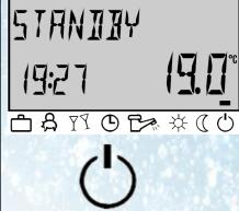
Heating and DHW are in standby. Frost protection is enabled.
