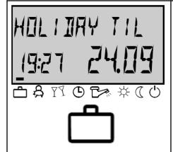
Vacation mode-Heating will be inactive until the specified date (this example is September 24). At 0:00 (midnight) on this date, operation will resume. This can be set 250 days in advance. DHW operation is set to freeze protection (100°F default).
