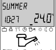
DHW only will operate based on the times and temperatures set in the "Timeprograms" chapter. If P1-P3 is selected, there will be up to three different schedules to choose. In this mode, heating will not operate—frost protection is enabled.
