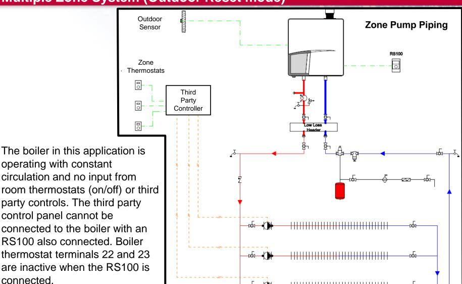
connected to the boiler with an RS100 also connected. Boiler thermostat terminals 22 and 23 are inactive when the RS100 is connected.
