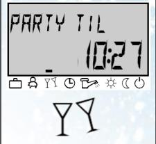
Party mode-Heating will remain in operation until specified time (this example is 10:27 am). This can be set between 0.5-24 hours OR if P1 is selected, heating will resume at the ON point of the next heating event.
