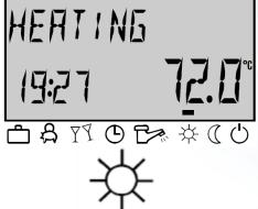
Continuous heating and reduced hot water operation according to temperature set points
