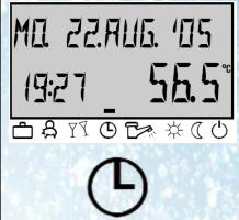
Operating Times-Heating and DHW will operate based on the times and temperatures set in the "Timeprograms" chapter. If P1-P3 is selected, there will be up to three different schedules to select.
