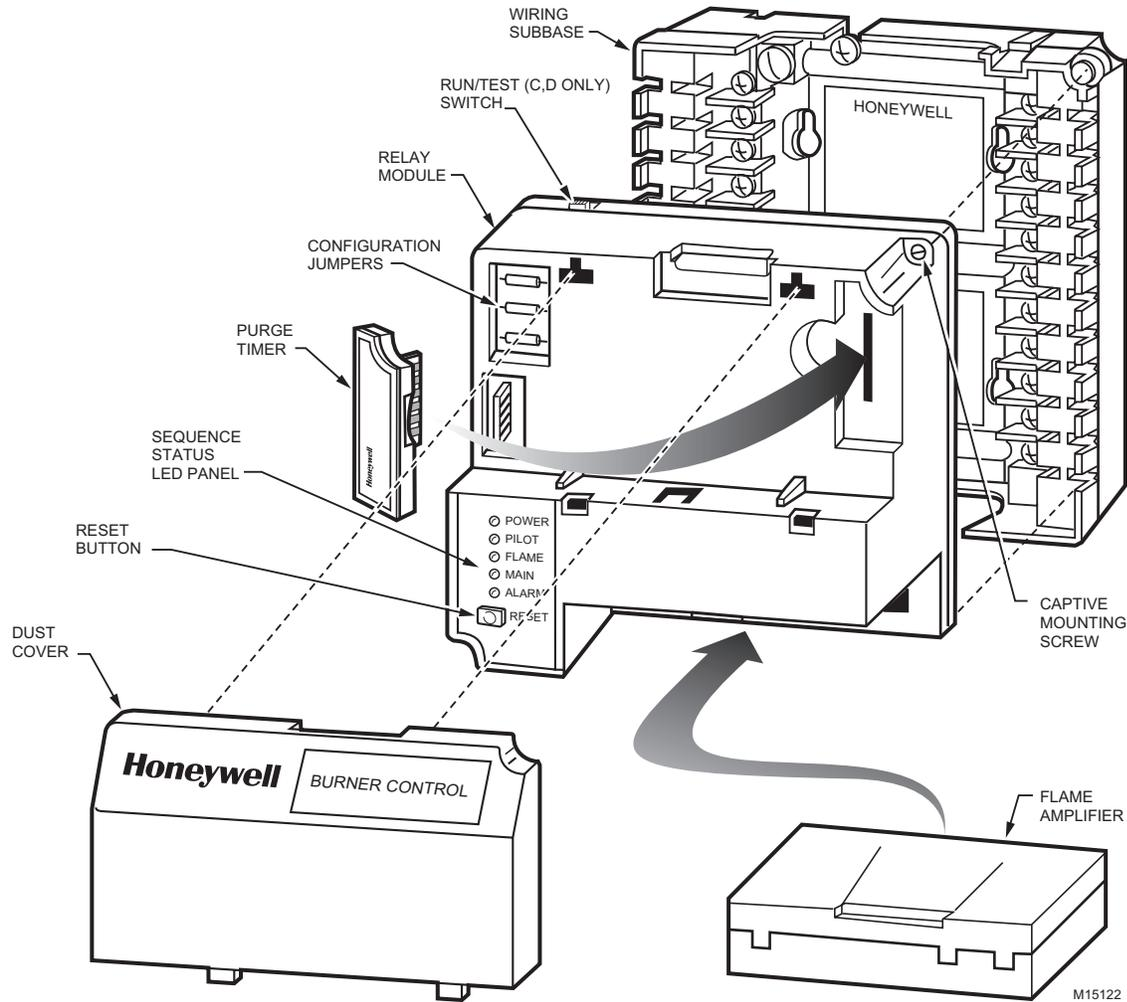
Fig. 4. RM7895A,B,C,D/EC7895A,C; RM7896A,B,C,D Relay Module, exploded view.
