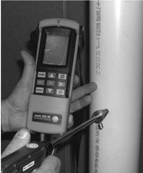
Figure 9.2: Insert Analyzer Test Probe into Test Port
