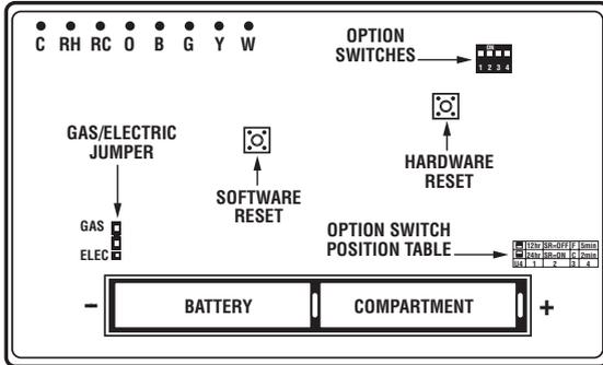
REAR OF THERMOSTAT WITH COVER REMOVED
