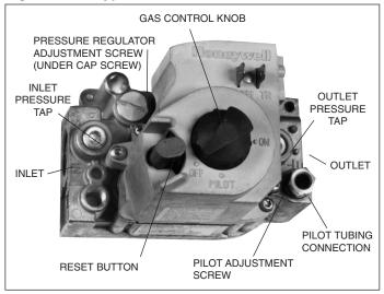
Figure 11.2 - Manifold Adjustment, Natural Gas
