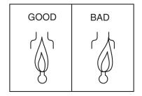
Figure 22.2 - Lifting Flame Condition
