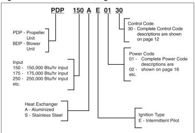
Figure 23.2 - Serial Plate ①
