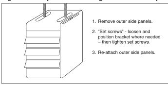
A pipe hanger adapter kit, shown in Figure 4.2 is available as an accessory. One kit consists of two drilled 3/4" IPS pipe caps and two 3/8 -  $13 \times 1-3/4$ " capscrews to facilitate threaded pipe suspension.
