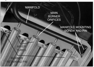
Figure 11.3 - Air Shutter Adjustment, Propane Gas
