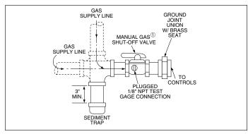
① Manual shut-off valve is in the "OFF" position when handle is perpendicular to pipe.
