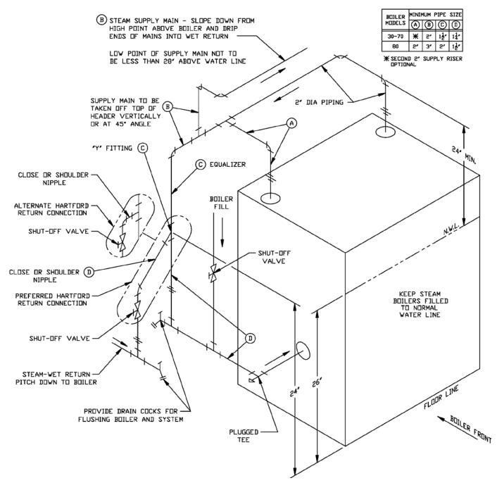
Figure 6: Recommended Boiler Piping for Gravity Return
