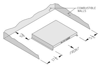
Figure 3: Special Base Installation
