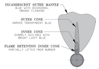
Figure 15: Main Burner Flame
