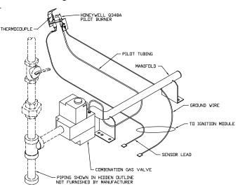
Figure 7: Pilot and Gas Piping, Intermittent Ignition (EI)
