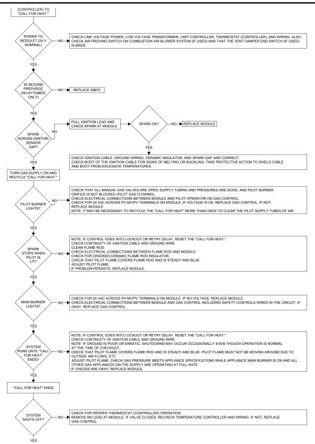
Figure 20: Honeywell Electronic Ignition Troubleshooting Guide
