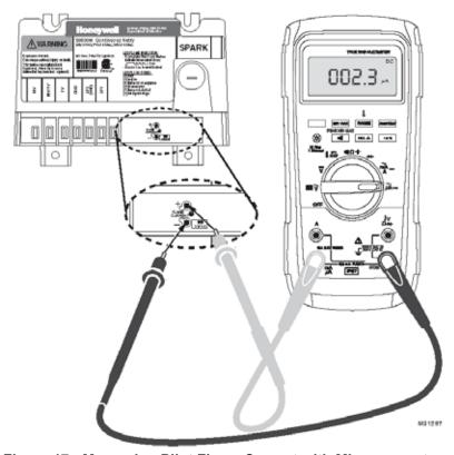
Figure 17: Measuring Pilot Flame Current with Micro-ammeter
