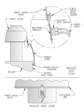
Figure 8: Blocked Vent Switch Installation
