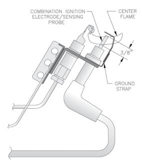
Figure 14: Pilot Burner Flame, Intermittent Ignition
