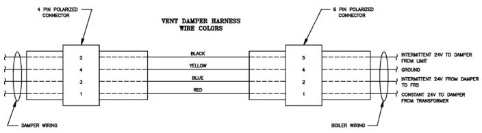
Figure 11: Vent Damper Schematic Wiring Diagram
