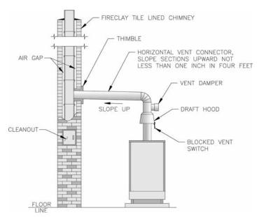
Figure 10: Typical Vent System Installation
