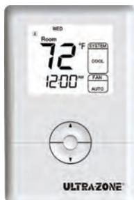
The Wireless thermostat with 7 day or 5 + 2 day programming allows for easy retrofit applications for zoning or non-zoning installations. The thermostat includes the wireless receiver and a wall mount bracket that allows for easy "pop-on" and "pop-off" for hand held programming. The EWT-3900 thermostat is compatible with Single Stage and Two Stage heating and cooling systems, as well as Heat Pumps and Three Stage heating and Two Stage cooling systems. The receiver will be 24V powered.
