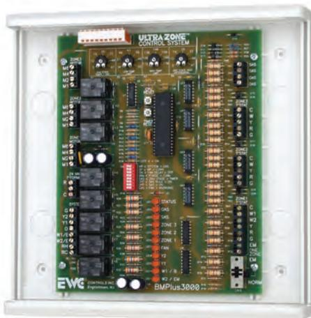
The BMPlus control panel is a single stage, two stage, dual fuel, and heat pump compatible panel controlling up to seven zones. The system features automatic changeover and fan control from any zone with a built in computer “watchdog circuit” to insure proper operation. The BMPlus is supplied with an SAS sensor for high and low temperature limit control that has field adjustable temperature limits.
