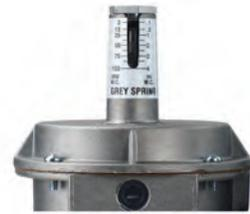
The EBD style by-pass are self-contained units that give you the static control mounted to the damper. It is an “all-in-one” design that makes the installation process much easier than most electronic by-pass dampers. The static pressure can be adjusted in the field between 0.1” to 4” of pressure. This is done by the turn of a set-screw. Requires 24VAC to operate. Tubing and pitot tube are included.
