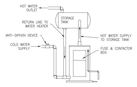
Figure 2 (Single Installation With Storage Tank Gravity Circulation)
