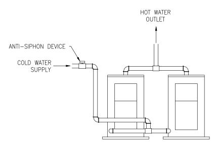
Figure 3 (Dual Water Heater Installation)
