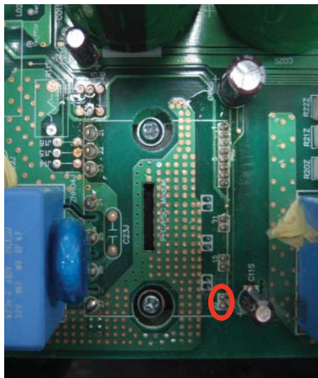
PFCM : Measuring resistance between No.19,20 pin
