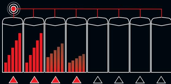
The "lead" boiler modulates with demand to capacity. As demand increases, additional boilers fire and modulate to capacity. This continues, with additional boilers firing and modulating to capacity until all units are operating. Every 24 hours, the SMART SYSTEM automatically shifts the lead boiler role to the next in the sequence, distributing lead-lag runtimes equally.
