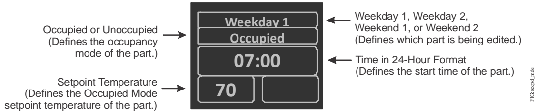
Figure 19: WT-4000 Series Pneumatic-to-DDC Room Thermostat Schedule Setup Screen for Occupied Mode
