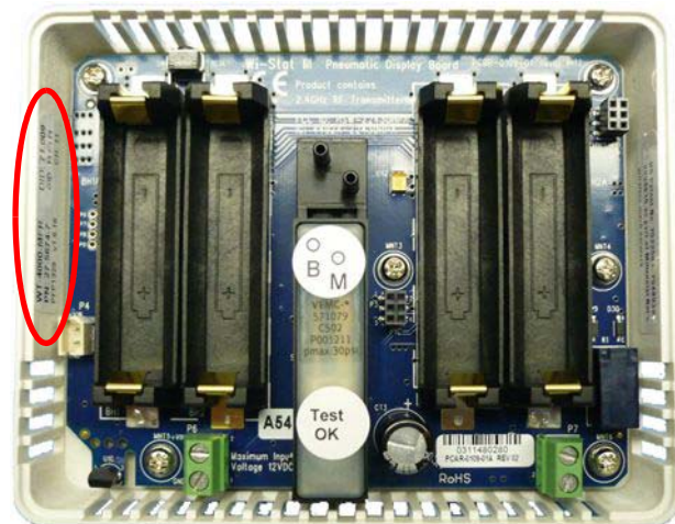
Figure 1: White Sticker on Inside of Room Thermostat Housing Showing Location of Group ID (GID) and Device ID (DID)
