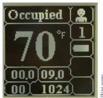
Figure 18: LCD during Stand-Alone Operation
