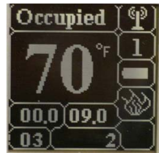
Figure 17: LCD during Wireless Communication
