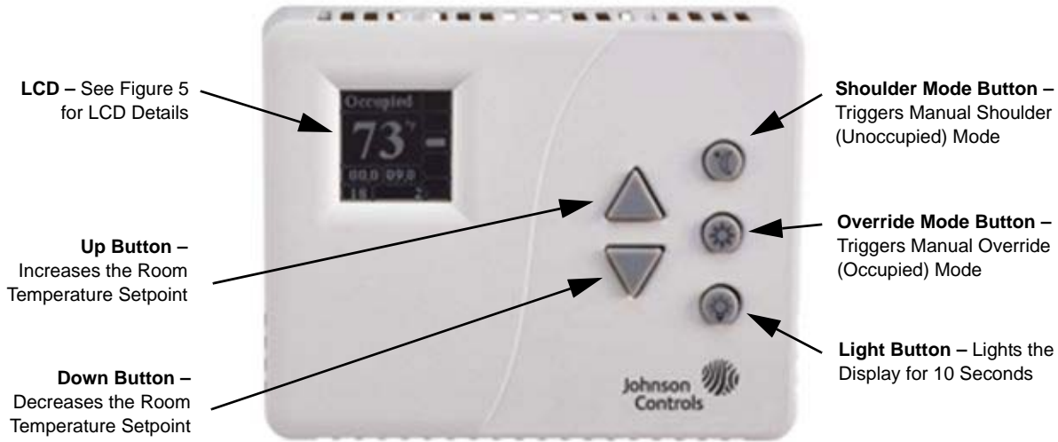
Figure 4: WT-4000 Series Pneumatic-to-DDC Room Thermostat Button Descriptions
