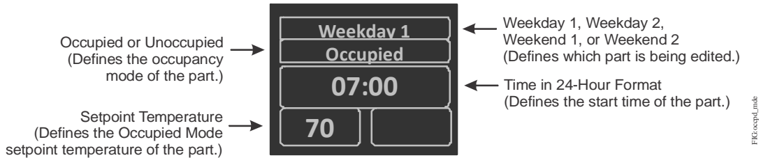
Figure 18: WT-4000 Series Pneumatic-to-DDC Room Thermostat Schedule Setup Screen for Occupied Mode
