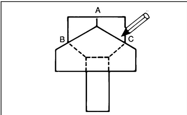
3. Place template so the corner is on the line below point A, and its edges are over points B and C. Mark new bend lines.
