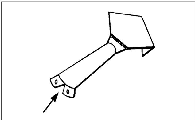
5. For Multi/Pak 80 only - front door may have to be flattened to fit. If so, notch flange bottom of front removing material.
