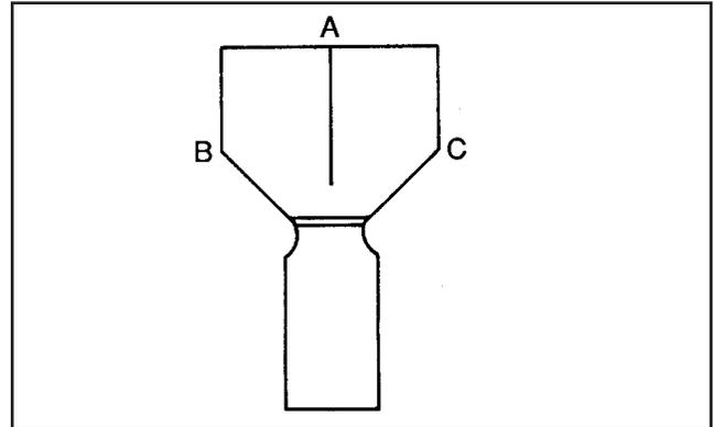
2. On the inside of the top corner piece provided, draw a vertical line from point A (center of top) down towards the hinge.
