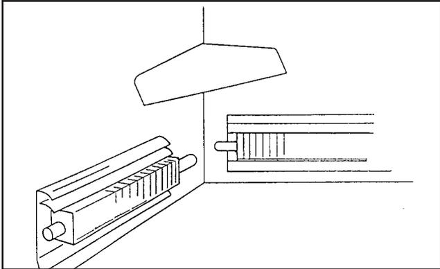
1. Using cardboard, cut a template to the exact angle of a corner.
