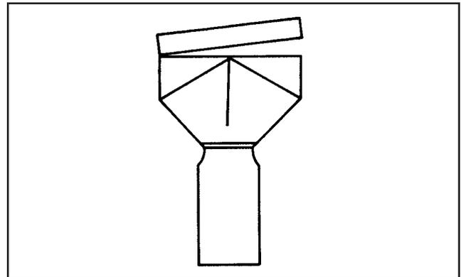
4. Cut off the portion above the corner of the new angle as shown. Bend flange along new bend angle.
