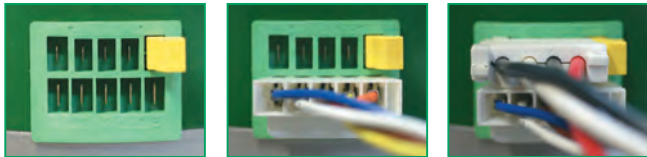
230VAC System Configuration (Yellow Jumper)
