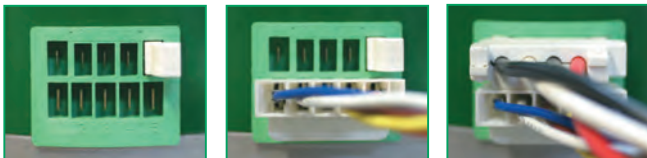
115VAC System Configuration (White Jumper)
