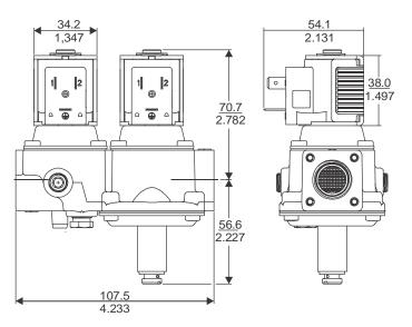
Figure 3: Bottom Adjust Regulator Dimensions, mm (in.)
