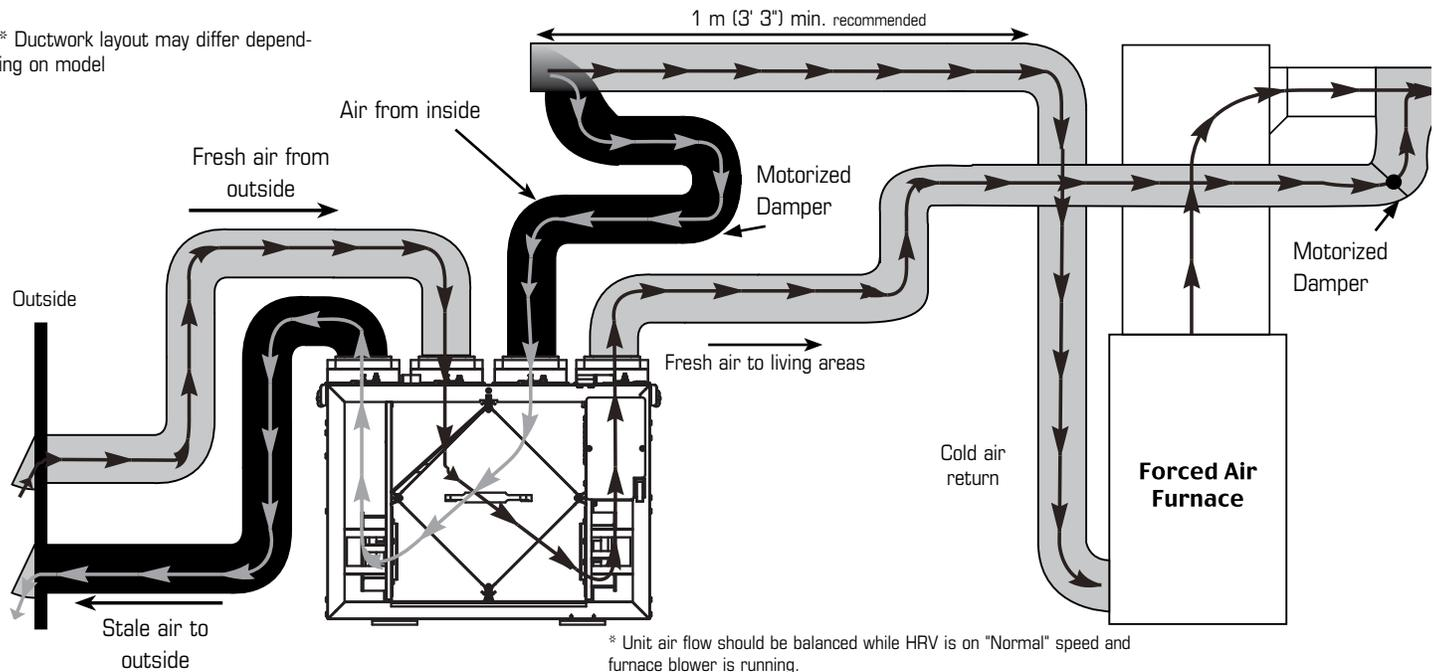
\* Unit air flow should be balanced while HRV is on "Normal" speed and furnace blower is running.
