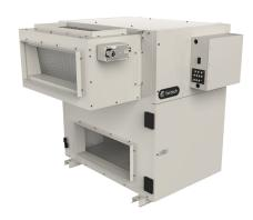
The SHR 8005R Commercial Heat Recovery Ventilation system (HRV) complements today's tight buildings. Fantech Heat Recovery Ventilators (HRV) are designed to supply air into a building while exhausting an equal amount of contaminated air to the outside. The aluminum heat exchanger core transfers sensible energy between air streams resulting in tempering of the supply air and reduced loads on the HVAC system.
