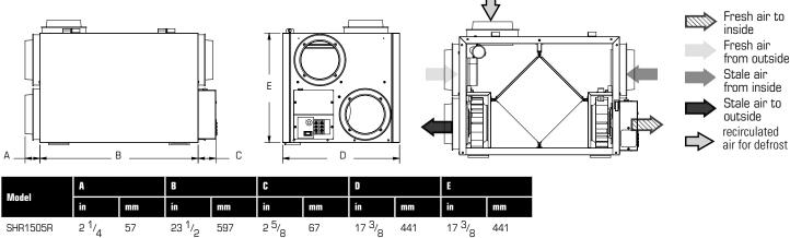
Clearance of 17" (432mm) in front of the unit is recommended for removal of core. All units feature three foot plug-in power cord with 3-prong plug.
