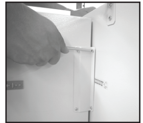
Figure 5 Bracket "B" tightened
