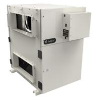
The SHR 14104 Commercial Heat Recovery Ventilation system (HRV) complements today's tight buildings. Fantech Heat Recovery Ventilators (HRV) are designed to supply air into a building while exhausting an equal amount of contaminated air to the outside. The aluminum heat exchanger core transfers sensible energy between air streams resulting in tempering of the supply air and reduced loads on the HVAC system.
