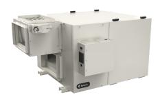
The SHR 11005R Commercial Heat Recovery Ventilation system (HRV) complements today's tight buildings. Fantech Heat Recovery Ventilators (HRV) are designed to supply air into a building while exhausting an equal amount of contaminated air to the outside. The aluminum heat exchanger core transfers sensible energy between air streams resulting in tempering of the supply air and reduced loads on the HVAC system.
