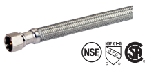
SS BRAIDED FAUCET SUPPLY 3/8 FIP COMP X 3/8 FIP COMP CHROME PLATED BRASS NUTS UPC/NSF-61 LEAD FREE
