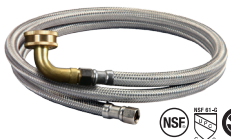
SS BRAIDED DISHWASHER CONNECTOR 3/8 COMP X 3/4 FHT SWIVEL ELBOW PVC TUBE, UPC/NSF, LEAD FREE
