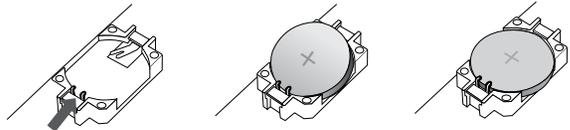
Slide the battery under the contacts and push down firmly
