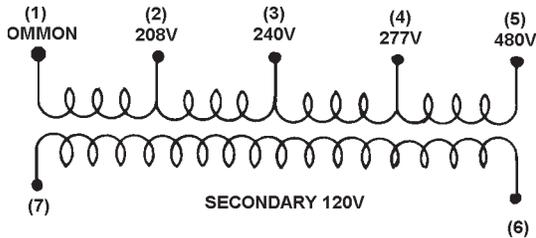
**IMMERSION THERMOSTAT MODEL TRANSFORMER**
