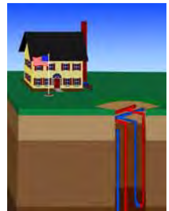
For a limited space, a vertical hole is used; this one shows two u-tubes.
