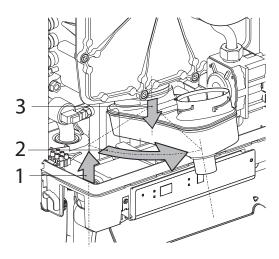
Fig. 25: Removal of Condensate Pan
