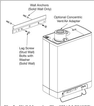
Fig. 2: Wall Mounting The CHALLENGER
