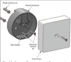
Fig. 22: Sensor Enclosure and Components
