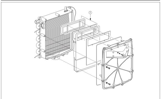
Fig. 32: CHALLENGER Burner Components
