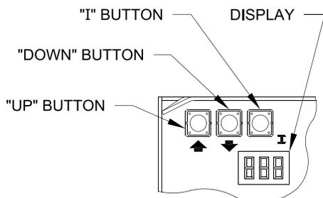
**Figure 30: Boiler Control Key Function & Orientation**
