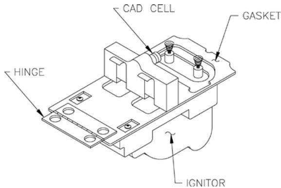
Figure 27: Cad Cell Location
