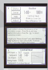
High resolution touchscreen display offers step-by-step assistance in setup and troubleshooting using text and intuitive menus, not codes.
