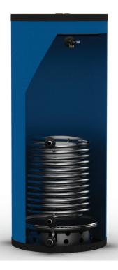
SST, the new stainless steel line of domestic hot water indirect tanks, feature important enhancements such as a welded and passivated stainless steel tank and heat exchanger, and two-inch thick, high-density insulating foam with a tested R value of 13.4. This new series of tanks offer capacities ranging from 40 to 119 gallons to suit all your hot water needs.
