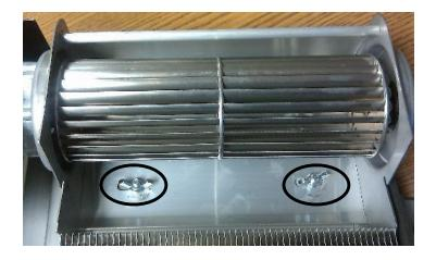
5. Remove 2 wing nuts holding blower in place.
