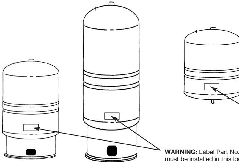
**WARNING:** Label Part No. 9015-463 must be installed in this location. If missing, it must be replaced.
