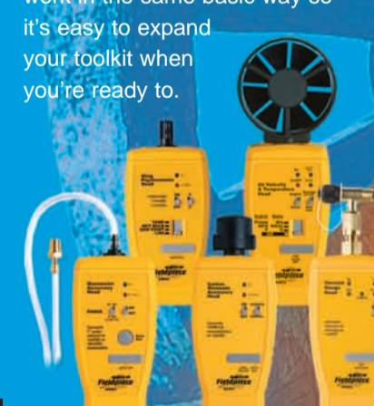
Fieldpiece accessory heads measure contact temperature (dual), IR temperature, RH%, wet bulb, dew point, dry bulb, air velocity, CO, milliohms, true RMS, high voltage, vacuum (vacuum gauge), gas and static pressure (manometer), pressure, superheat, and subcooling.
